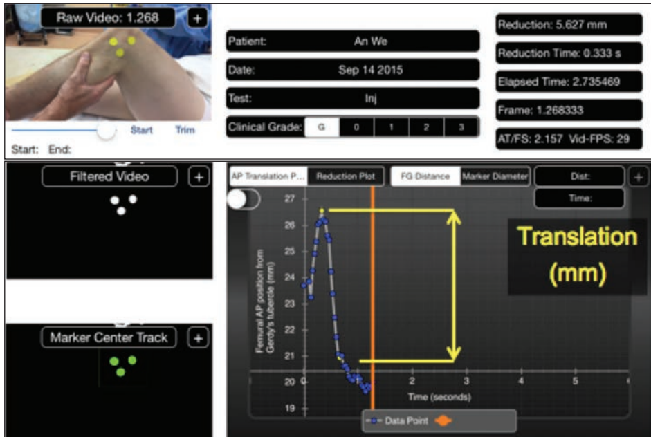
Fig. 4: Configuration of skin markers and display of software interface for PIVOT application for the I-pad. A pivot shift test is performed in the photograph on the upper right with skin markers placed on the lateral femoral condyle, Gerdy's tubercle, and the fibular head. Tracking of the skin markers as observed on the iPad interface are shown in the two lower left boxes prior to and during the performance of the pivot shift. The change in the anterior-posterior position of the femur in relation to Gerdy's tubercle is recorded as a function of time as observed in the lower right image. The lateral compartment translation during pivot shift test was calculated by subtracting the highest and lowest values along the graph, which in this case is 5.627mm.
