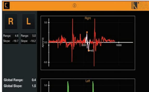
Fig. 3: Screenshot of the Ipad showing acceleration plot for right knee during pivot shift testing, created by Image sensor technology Kira (Orthokey LLC, Lewes, DE, USA). White highlighted part in the curve shows the points of maximum and minimum acceleration. Acceleration range is calculated by subtracting minimum acceleration from maximum acceleration. Higher recorded peaks that occurred after pivot shift phenomenon are due to the sudden full extension of the extremity.
